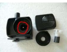
Then rinse everything, being very careful not to bend or damage the impeller axle (circled in red in the picture). If very slimy or calcium encrusted, soak in a 1:10 solution of vinegar and water.
