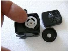
Take off the grid, underneath is another black cover with a round hole that you can pull off, making the white impeller visible. Gently remove the impeller making sure not to bend or damage the white plastic part. Hit the pump against your hand so that anything that might be lodged inside has a chance to come out.
